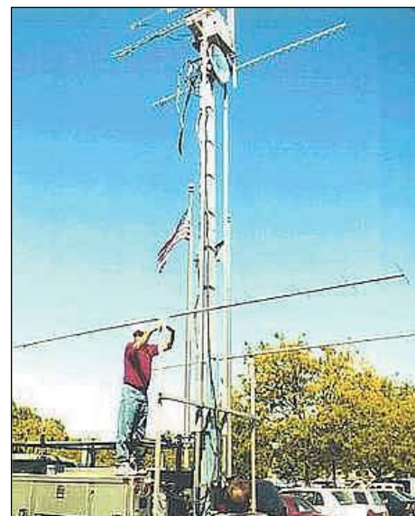
KA1ZE's portable VHF-to-microwave station.
