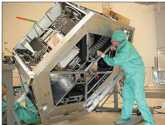
Putting the bottom plate on Phase 3-D.
