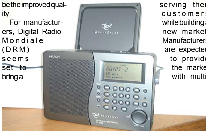
The Hitachi EH-WS1, an MW, SW (broadcast bands), VHF/FM, and WorldSpace digital satellite receiver. The small satellite antenna that receives the WorldSpace service can be unclipped and positioned within sight of a satellite. When deployed separately, the handle serves as a stand for the satellite antenna, a 5m-long extension lead (included) connecting it to the receiver.
