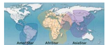
Fig 1: Footprints of the three beams of the Afristar, Asiastar and Ameristar satellites. The beams carry differing program contents to different areas of the globe.
