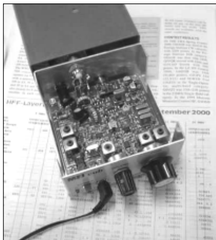
The MFJ Cub: wiring done, now just to put it in its box.
