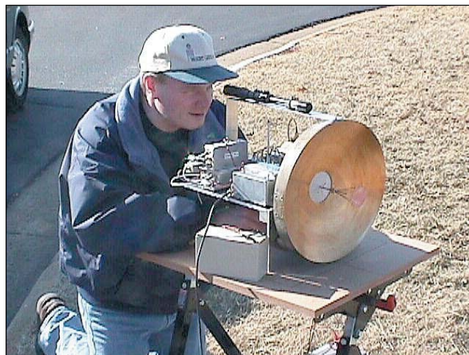
Taking aim: WA1ZMS aligning the 145GHz dish using a gunsight.
