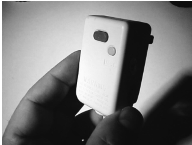
You can get a circuit breaker in a rocker switch, you can get a circuit breaker in the style of an automotive blade fuse, and now you can get a circuit breaker in a power plug... so long as you use 110V mains.
