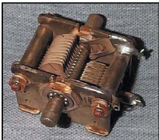
A variable capacitor. The capacitance is changed by varying the area of overlap between the fixed vanes and the rotating vanes.
