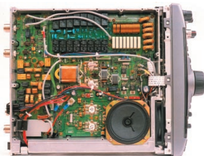
Top view with covers removed showing PAs, filters and ATU.
