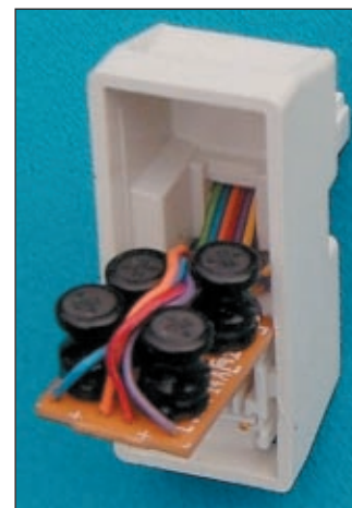
The BT 'Freelance' LJU10/14A telephone RFI filter for frequencies up to a few Megahertz.
