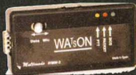
If you want to receive data, then connect the audio output of your receiver to the WMM-3 and the output of the modem to your PC serial socket. A CD-ROM is provided with lots of software, this will get you started.
