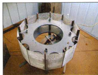
Brian, CT1DRP, has had trans-Atlantic success using this superb coil wound with aluminium wire.
