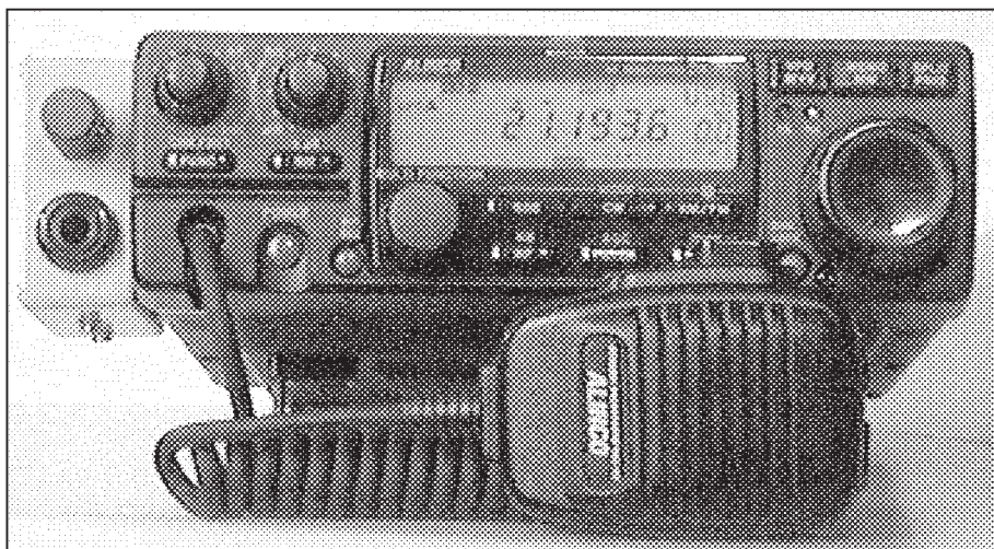
The Alinco DX-70TH with the power controller in position. It presents the operator with a handy extra control.
