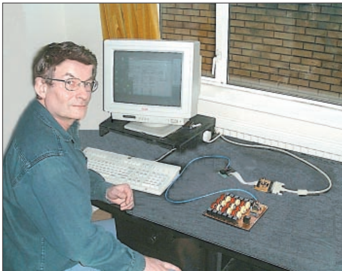
The IT Department in the author's shack. On the desk is his LPF board connected by umbilical to the TOPIC programmer. The parallel port cable can be seen disappearing off to the PC.
