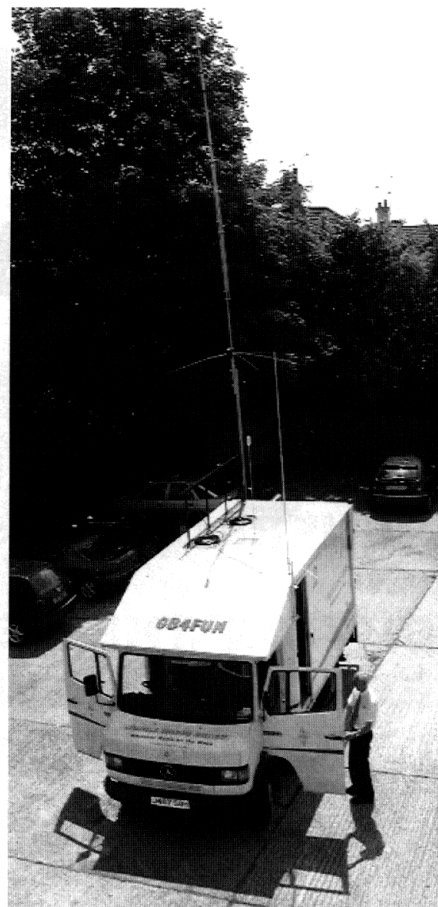
The roof showing the handrail, the R-6000 vertical atop the telescopic mast, the 7MHz whip (centre) and the VHF / UHF collinear (front nearside).
