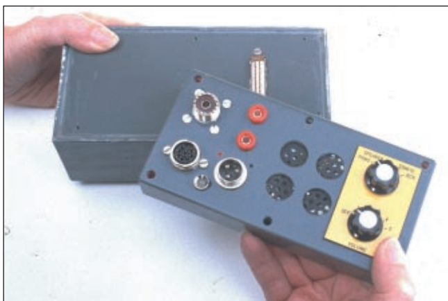
The sealed bottom box contains the electronics, all connections being made via a single 25-way D-type connector to the top box, which contains damage-prone components.
