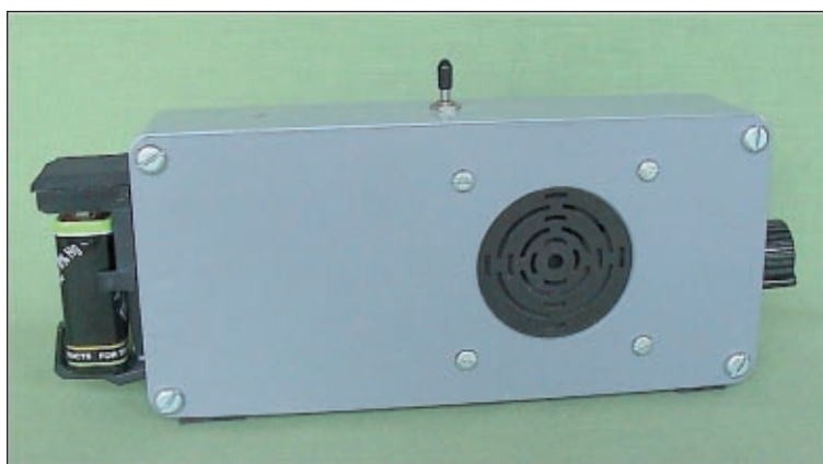
The battery-powered version of the Sonic Wattmeter.
