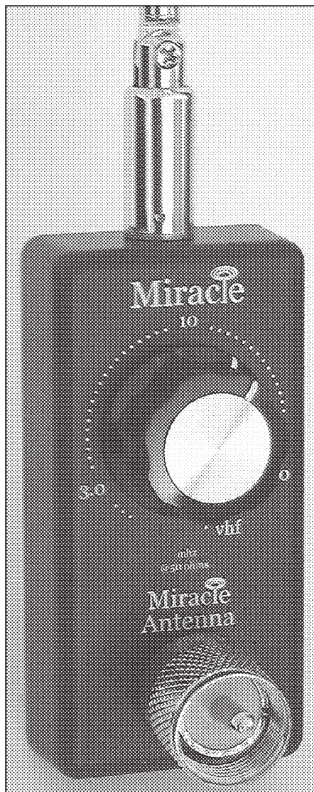
The 'Miracle Whip' matching box. Its size can be judged from the PL259 plug.
