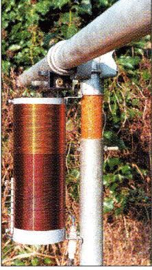
Simple modification to allow LF top feeding by changing the feed cable between LF tuning coil and HF balun.
