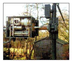
The upper part of the author's top-fed antenna, tuner open and tower luffed. It provides allband coverage, 1.8 to 30MHz at full power, with tower at any height. The photograph shows the insulating plate with HN output connector, Tufnol rod insulator and HF balun. The vacuum relay is hidden between the variable inductor and ceramic variable vacuum capacitor. The 'sardine tin' (top left) contains silica gel desiccant.
