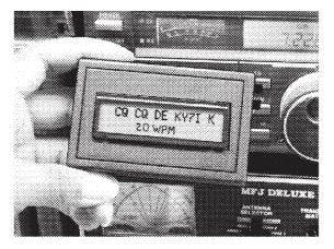
cycled through by pressing and holding the button in for more than two seconds. In Modes 1 (the default) and 3, the speed of the received Morse is displayed all the time, but doing so means there is less room to display received Morse - 24 and 16 characters respectively. In Modes 2 and 4, which differ in the way that characters scroll across the screen, a maximum of 32 characters can be displayed.
