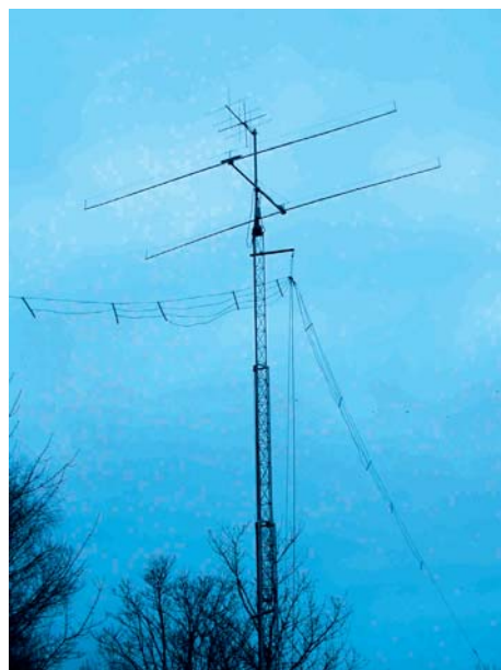
The GB2CPM multiband dipole, configured as an inverted-V on the 7, 10, 14 and 18MHz bands and each dipole can be tuned without any noticeable interaction. All the other operators are very pleased with it.
