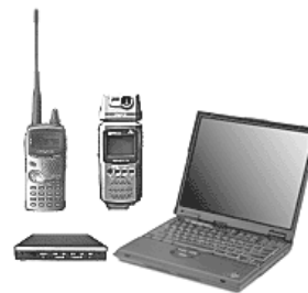
The complete transmit and receive SSTV system: the Kenwood TH-D7E, VC-H1, TNC and laptop.
