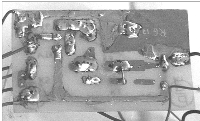
Underside of the circuit board. The design is quite suitable for construction on matrix board, because the layout is not critical.
