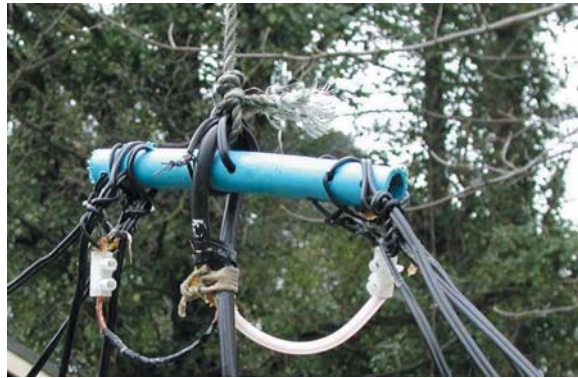
The plastic tube centre insulator for the GB2CPM multiband dipole
