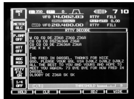
Top: LCD panel showing spectrum display. Above: LCD panel showing RTTY decoder display.
