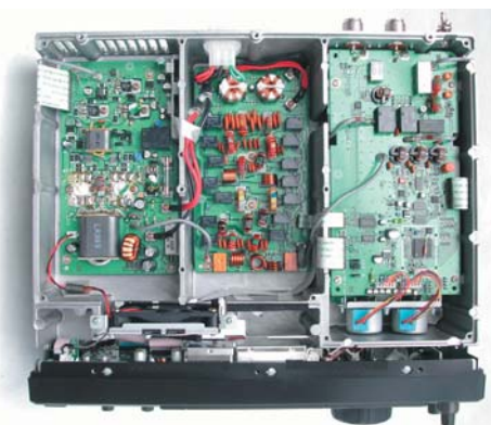
Top view with covers removed showing PA, filters and ATU.
