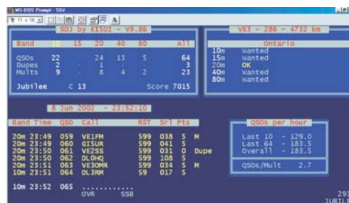
Fig 2: The main logging window of the SDJ program by E15DI, showing Summary Score Window, Country (VE3) Worked / Wanted Window, Logging Window and QSO Rate Window.
