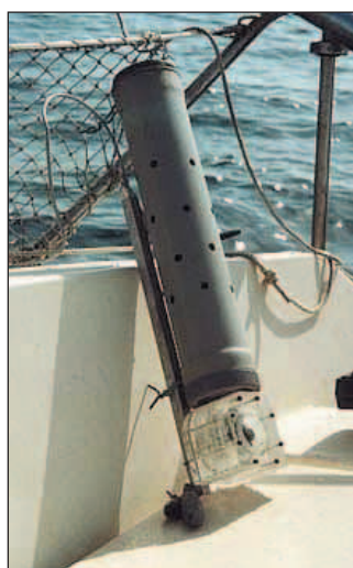
The camera is attached to a perforated cylinder which is filled with crushed sardines in order to attract the underwater ATV stars, some wanted, some not (see later).
