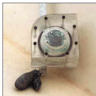
A small black-and-white TV camera sealed in a home-made plexiglass box, with O rings. It is connected to a screened cable with three conductors: video output, 12V supply, and common. The cable measures 17 metres, the maximum operating depth. (Photos: F5AD)
