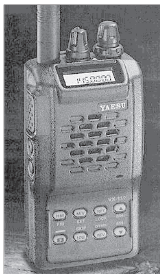
The VX-110 from Vertex (Yaesu), a commercial-grade VHF transceiver that is programmed for the 144MHz band and sold in France into the amateur market. A sister model, the VX-150, is also available.
