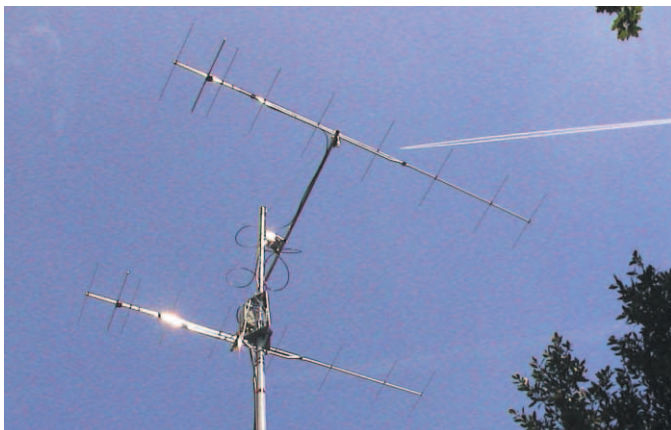
This is the new 2m array at Niels Montanana's, G8RWG, QTH. The two Yagis are 9-element, 2-wavelength antennas to the DK7ZB design, 12m above ground. He hopes to try some EME skeds using JT44 software.
