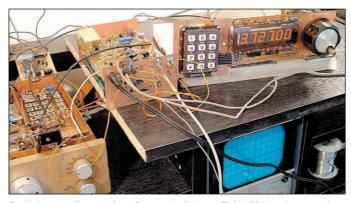
Early integration testing. Bottom left is my Third Method transceiver (borrowed front-end and PA), top right is Pic 'N' Mix DDS still on its original breadboard (injection and controls) - and in the middle is the new DSP module. Note that Pic 'N' Mix provides all the transceiver controls, leading to a clean and compact front panel.
