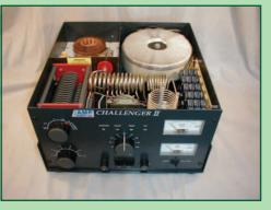
The new CHALLENGER II uses a GS35 triode to produce 1500W on all bands,
