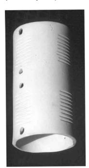
The coil former before firing. All holes have been drilled and wire guide-grooves cut.
