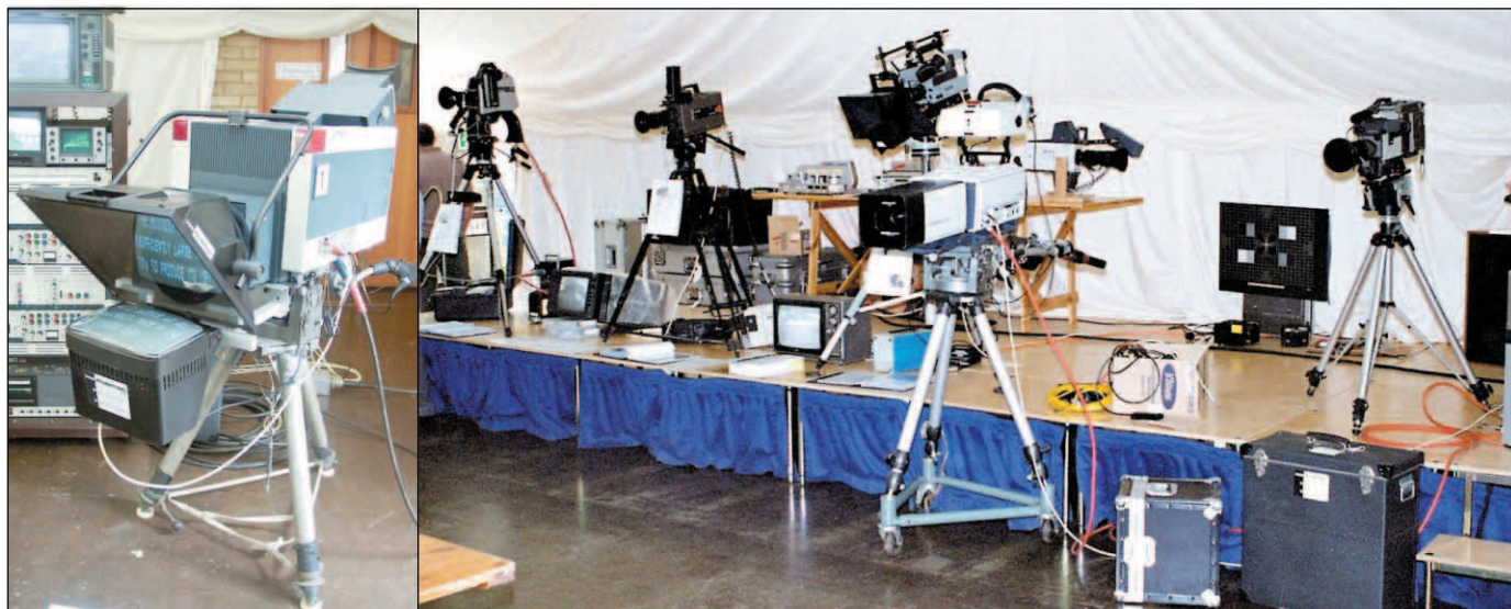
Left: a Link 110 camera; right, a selection of cameras, including a Philips LDK90 and LDK14, and a Link 130 and 120, all courtesy of Paul Read.
