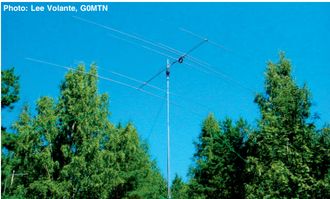
The WRTC2002 beam: a 6-element tribander with two elements on each of 10, 15 and 20m, made in Finland especially for the event.
