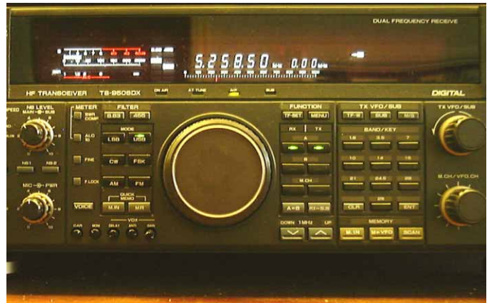
How to set up an SSB transceiver for 5MHz-band operation. Note that USB (not LSB) should be used and that the VFO should be set 1.5kHz below the spot frequency, so that the centre of the transmission is on the nominal frequency (in this case 5260.0kHz).
