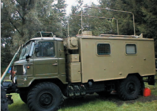
Russian army radio communications vehicle, with two NVIS magnetic loop antennas mounted on the roof.
