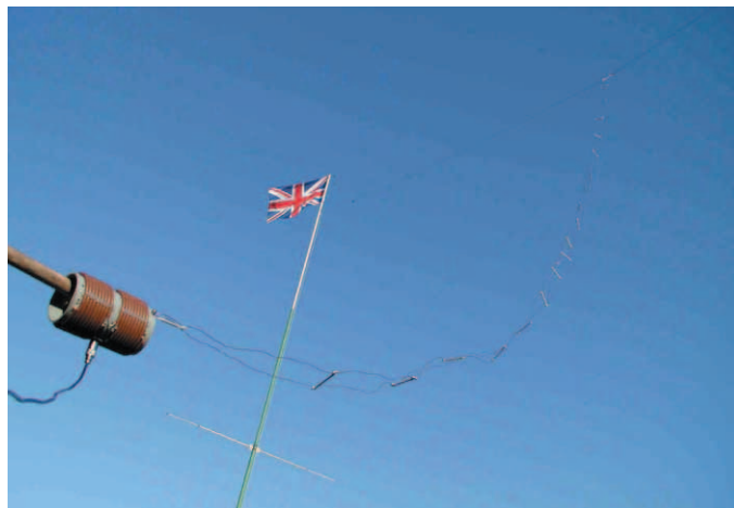
The 50ft length of wire centre fed with home made twin-line feeder. In the foreground is a PA0SE coax balun. This arrangement was replaced with 450Ω ladder line all the way back to the outside of the shack, with a short length of coax through the wall to the ATU.
