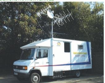
THE GB4FUN amateur radio demonstration vehicle now sports some additional antennas. Thanks to a generous donation by AMSAT-UK, GB4FUN is now fully satellite-capable. The new antennas include 2m and 70cm cross-polarised Yagis, plus a 2.3GHz dish with down-converter to 144MHz. The antennas are rotatable and tiltable, and can be computer-controlled to track the satellite as it passes overhead.
