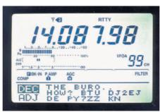
MUCH OF THE operation of the IC-7400 centres on the monochrome LCD dot matrix panel and associated five function keys along the bottom, as used in the IC-746. The upper part of the panel displays the frequency, mode, RIT offset, memory, antenna etc and status of all selected functions. A bargraph meter displays signal strength, power output, ALC and SWR with optional peak hold.
