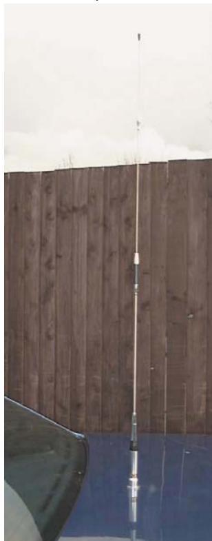
The Apex, Exceed and SHG series of VHF / UHF verticals all have the same PL-259 screw fitting.
