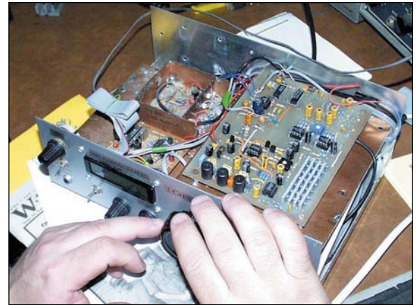
The QRP2001 multi-band HF receiver.
