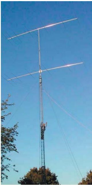
Mike G3SED's stacked pair of Trident ® 6 mtr 7 element Long Boom Yagis - spaced 22ft at 75ft high
