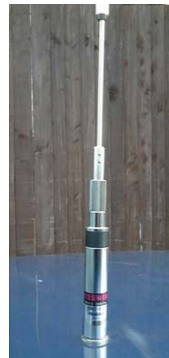
"More chrome than a 1959 Cadillac"? Close-up of the Maldol SHG for 144 and 432MHz.
