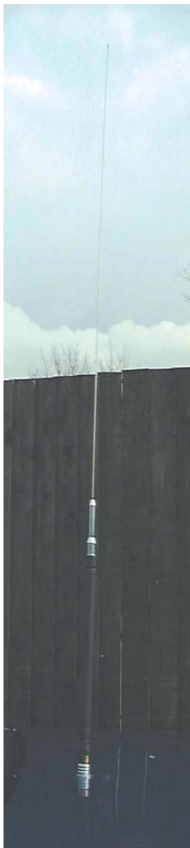
The HFC monoband antenna, with 80m coil attached.
