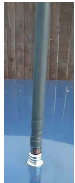
Close-up of the HFC 80m loading coil attached to the top of the car boot.
