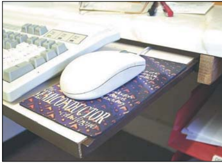
Kitchen drawer runners make a strong pull-out support for a keyboard below the desktop.
