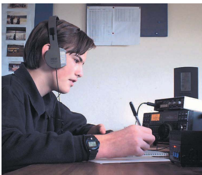
Jonathan, M5FUN, has 'fun' operating on HF with this simple station: a 100-watt transceiver powered from a 13.8 volt mains power supply.
