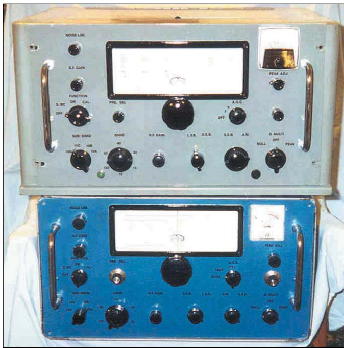
Two excellent examples of the classic G2DAF HF receiver. Top, the receiver built many years ago by the late GM3AVA in consultation with G2DAF and now acquired by G8HLJ. Underneath is G8HLJ's recently-completed model using similar screened wiring techniques.
