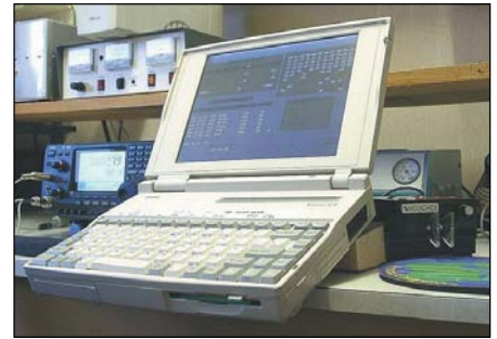
Tilting a laptop PC off the front of a table, to make the keyboard more comfortable. Note the compact layout of radio, laptop and keyer, all within easy reach.
