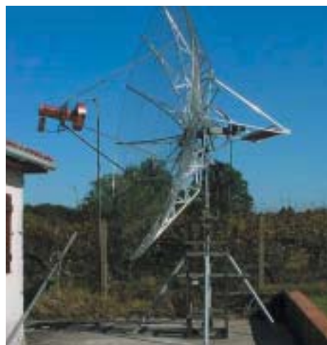
This is the home-built very lightweight 3.95 metre dish for EME work constructed by Graham Daubney, F5VHX (formerly G8MBI) (JN04).
