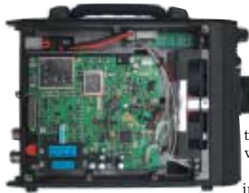
Under the top cover of the FT-897.
