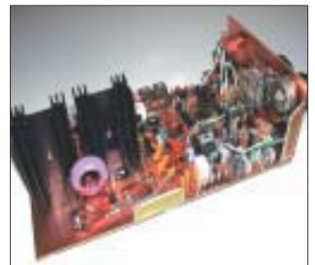
The Walford 'Fivehead' transceiver with the Linear amplifier attached.
