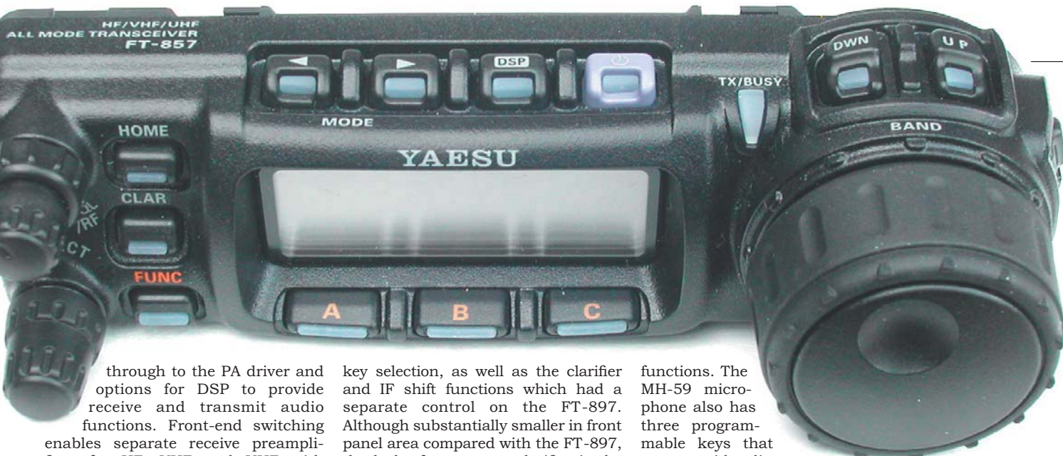
Above: The FT-857 has a detachable front panel.
