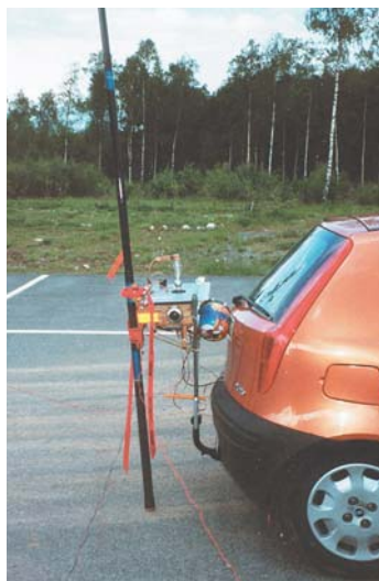
Left: The SM6FLL clip-on antenna mounting panel and matching/loading unit fixed to the vehicle using a bicycle carrier frame mounted on the tow-bar.
