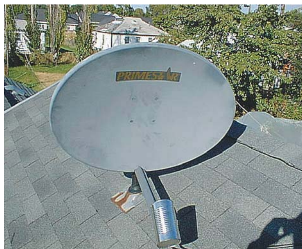
A satellite TV dish adapted for use as an IEEE 802.11b antenna. Being an offset dish, it needs to be angled down when pointing towards a target on the horizon. This arrangement is quoted as providing a gain of about 22dB at 2.4GHz.
