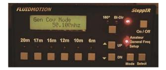
Top: Close-up of the Controller unit, showing the unique 'Normal' / '180°' / 'Bi-Dir' control.
