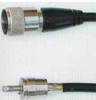
Coax cable preparation prior to fitting to the plug. Note the clockwise twist in the centre conductor.
