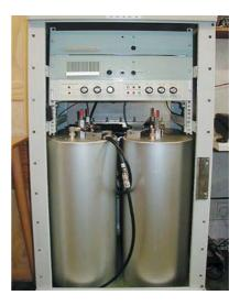
GB3DX cavity filters, control logic, receiver and transmitter.
