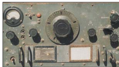
The 1942-43 Australian AMR100 (US SC-CD-136.43), replicating the HRO, but using glass-octal valves (6U7G, 6J7G etc).
