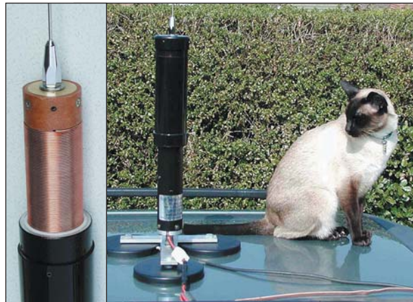
The variable inductive loading of the High Sierra Sidekick shown with weather protection shield removed. The coil is moved in and out of the lower tube with a motor-driven lead screw.
