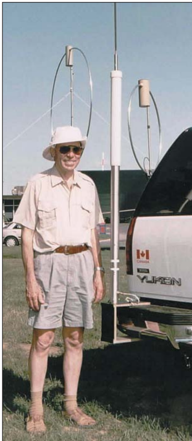
Two compact loops, the AMA 7 and the AMA 8 (3.4m and 1.7m-diameter loops) and the author's tunable all-band (TAB) mobile antenna, in operational use during a simulated emergency communications exercise.
