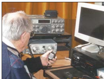
Ray Rogers, G3LIA, a bhi NES10-2 noise-eliminating speaker sits on top of his TS-930S transceiver.
