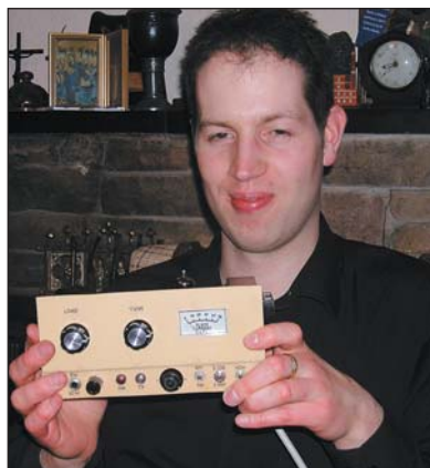
Hans Summers, G0UPL, shows off his valve CW transmitter for 40 and 80m to G QRP Club members after the last Rochdale QRP Convention.
