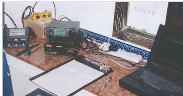
The CN2PD set-up at the Hotel Tikida Garden, Marrakech. The IC-706 sits on top of the Watson W-25SM SMPSU, with the MFJ-901B ATU to the left. Note the lightweight CW paddle key fixed to the clipboard.
