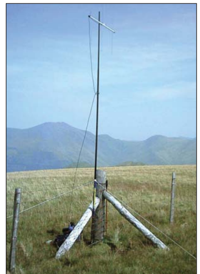
Centre SOTA Beam ready for SSB (horizontal) use from GW/NW-020 Craig Cwm Silyn on the Nantlle Ridge.
