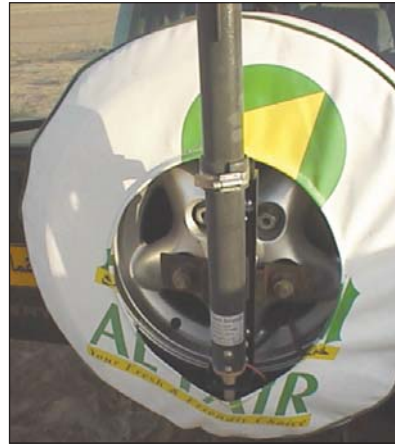
This is how A45WG/M solved the problem of mounting the antenna to the vehicle.
