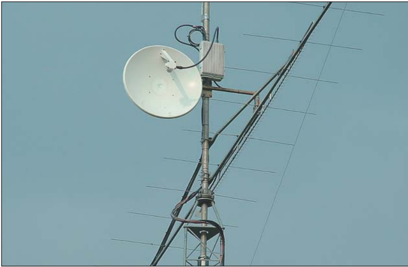
The 60cm prime focus dish used on 5.7GHz by G4PBP. This is a commercial Stella Doradus dish and feed, modified by Russ to optimise its performance within the 5.7GHz amateur band. The masthead transverter and power amplifier can be seen beside the dish.
