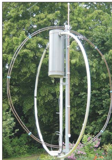
AMA5 (CapCo) 1.7m loop with two turns and HV tube capacitor for 160m.
