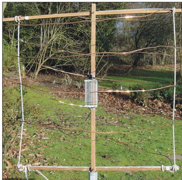
Five-turn 'coil' (1m x 1m) for 160m and 80m.
