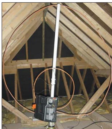
Multi-resonant 3.5 to 30MHz rotatable 1.4m loop in attic.
