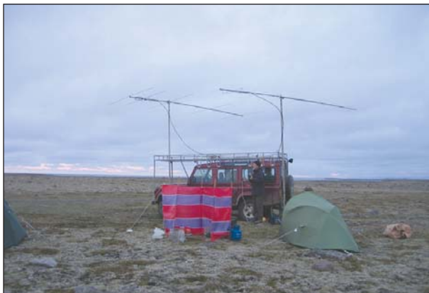
This is Keith Tatnall's, G4ODA, mobile station set-up just 2.5km south of the Arctic Circle in Iceland on 19 June in IP26. The Yagis are for 2m and 6m and that's Paul Bradfield, G1GSN, standing by the vehicle.
