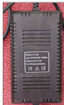
p56 – Switch-mode battery charger
