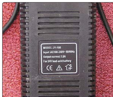
A switch-mode battery charger for electric scooters.
