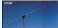
Don't want a wire antenna but can't fit a Yagi, then consider a rotatable dipole.
