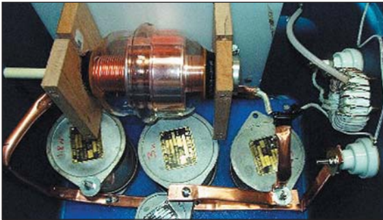
The ATU of Laurence, WD2XDW, built in a stacking box. You can see the 'doorknob' capacitors below the vacuum variable.
