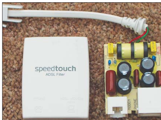
p70 – An ADSL filter tested. See 'EMC'.
