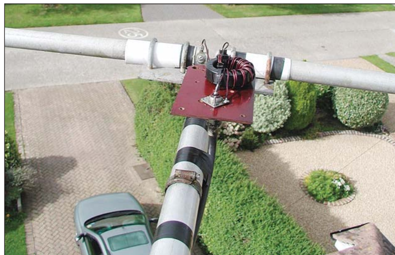
Seagull's eye view of the current balun fixed to the feed-point of the modified MQ-2, before the protective grease coating was applied.
