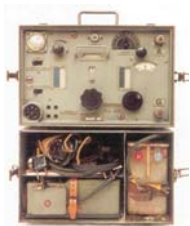
G4PRI's German Torn E.b TRF mechanically-elegant backpack receiver with large turret coil assembly, as illustrated on his QSL card.
