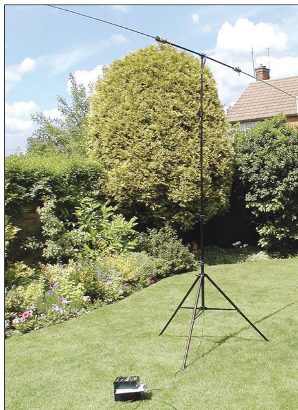
The erected Buddipole, with optional mast and tripod. Notice the very small amount of element droop at full extension.
