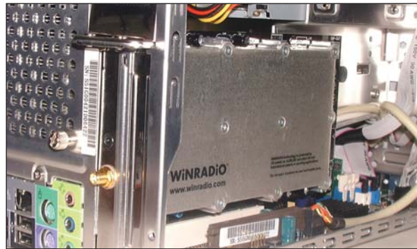
The G313i is a plug-in PCI card with an SMA antenna socket and audio output socket provided
