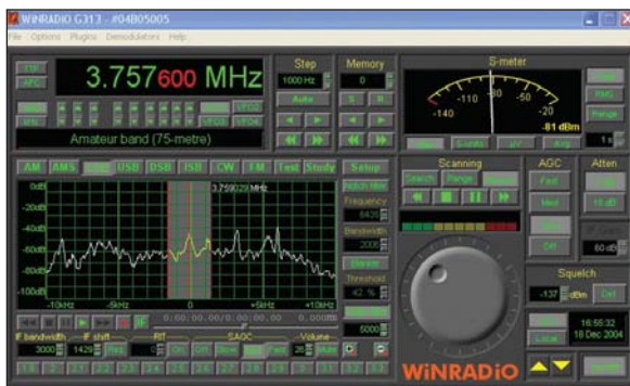
Above: The main receiver panel display, showing the selected signal frequency and IF bandwidth.
