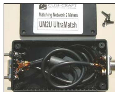
Left: Cushcraft employs a half-wave balun made from coaxial cable, plus a ferrite tube to prevent RF flowing back down the braid of the feeder.
