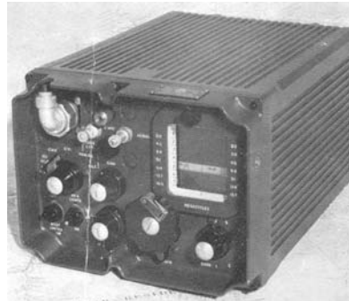
Top to bottom: The Russian Volna-K maritime receiver covering 12kHz to 23MHz with gaps in nine bands. Single conversion with IF 85kHz up to 600kHz and double-conversion with IFs of 915kHz and 85kHz above 1.5MHz. Optical projection calibration scale.
