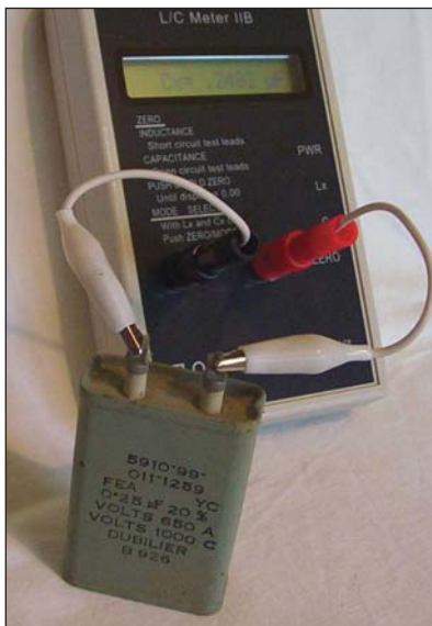
Above: An old paper capacitor of nominal value 0.25µF.
