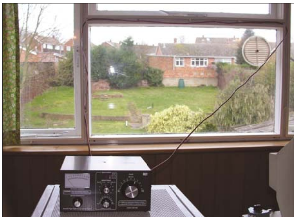
Above left: The 12ft wire loop mounted on the PVC spreaders on top of the MFJ-936 ATU.
