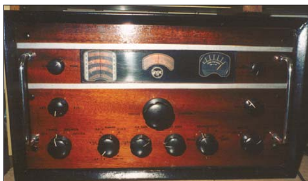
The restored RCA AR88D. This receiver is far from being in original condition, with its first RF stage replaced with an miniature EF183 valve and its metal cabinet replaced by a wooden one, made from Western Australian jarrah. However, it works well and is a great talking point.
