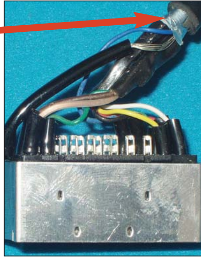
Right: A standard type of SCART cable with shielded signal cables and an overall foil shield (arrowed).
