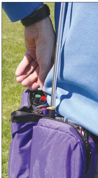
Photo 3: The uplink transmitter located on my waist, with pan, tilt and shutter controls beside my hand. The aerial extends up my back where it doesn't obstruct kite-flying.
