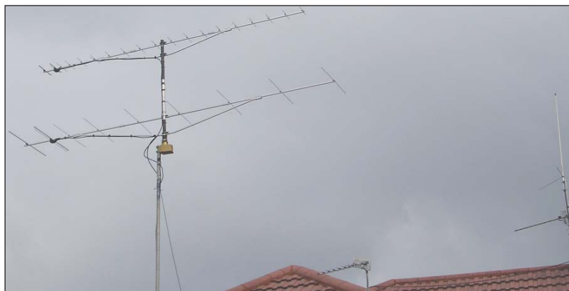
This is Ian Hogan's, G6TGO, VHF/UHF Vargarda antenna installation showing the 19-ele 70cm Yagi above the 9-ele 2m one.
