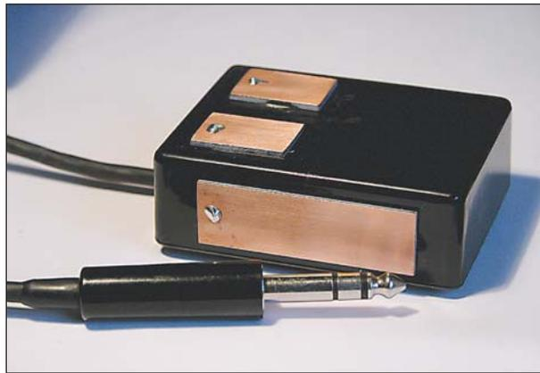
**The new Piano Keyer, showing the dot pad on the top left and the dash pad on the top right of the box, with the earth pad on the left-hand side of the box. There is an identical pad on the opposite side.**
