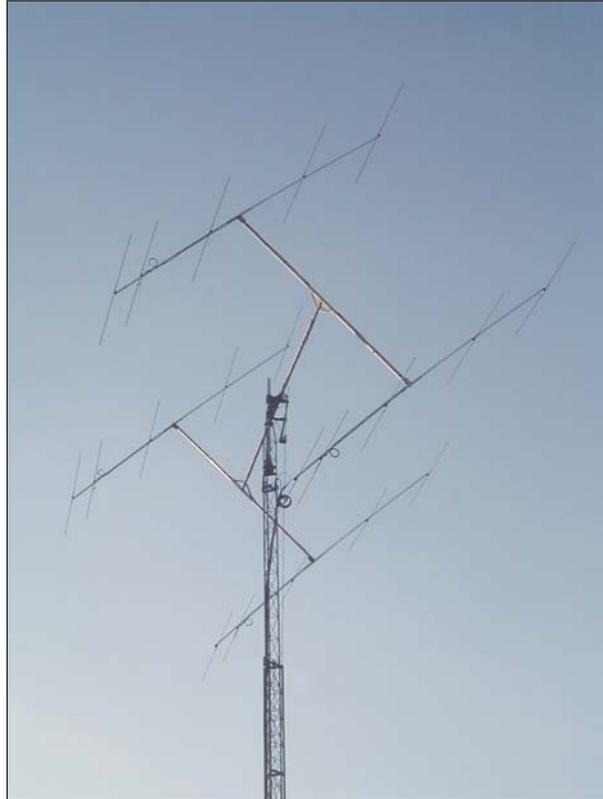
This is the 15.1dBd gain 6m EME antenna array designed and built by Ian Williams, MOBCG, which he used to make the first British Isles to New Zealand and Alaska QSOs. The four 5-element Yagis have 22ft booms and are mounted on an H-frame. The elevator is steerable from 0° to 90°.
