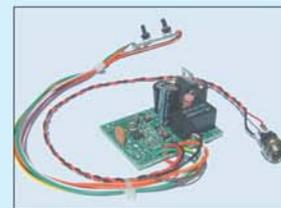
The NEDSP1062-KBD comes with the fitting kit, labels, fused DC power lead and installation instructions.
