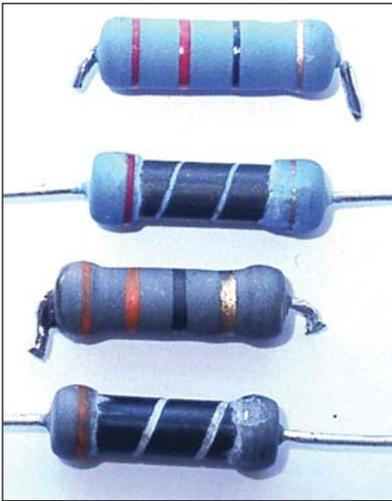
Metal film resistors revealed. The dark material is the metal film, and the light helix is the underlying ceramic.
