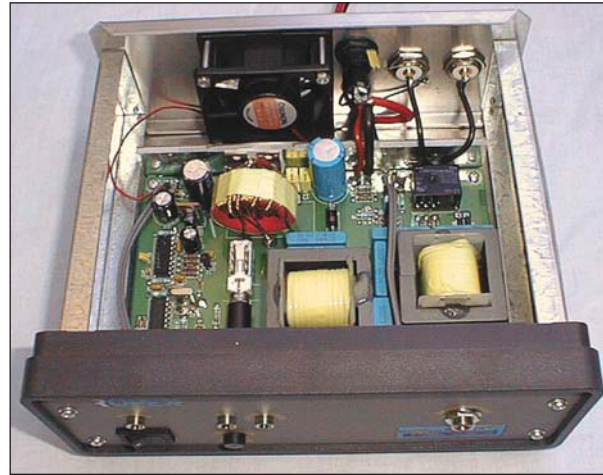
The Ropex transmitter exposed. The crystal can be seen next to the chips on the left.
