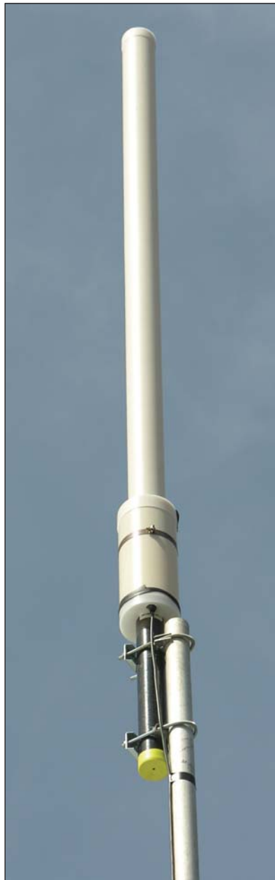
An alternative method of mounting the E-H antennas: directly on to a 1.5in dia pole.
