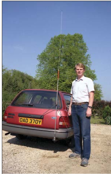
Author G3TSO with 80m mobile installation.
