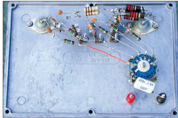
My 3M impedance measurement bridge showing its simplicity. This model, built in 1970, is still going strong.
