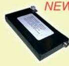
One-Plug Power is the internal FT-817 battery solution you have been waiting for until now. One-Plug Power comprises a 1900 mAh NiMH battery pack, both over-temperature and over-current protection, connection to the FT-817 Molex connector, and a modified Yaesu battery cover door featuring a power jack that allows connection of a battery charger such as the Maha MH-C777 or MH-C888.
