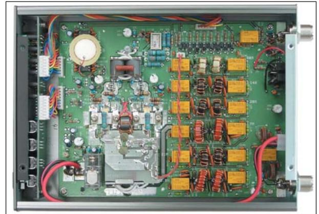
similar to the smaller amplifier and, according to the Tokyo Hy-Power website, the amplifier is suitable for CW QSK operation. Two antenna sockets are provided on the rear panel and a front-panel switch selects between them. An auto position will automatically select antenna A on HF and antenna B on 50MHz even with the amplifier turned off, providing it is still connected to the mains supply.
