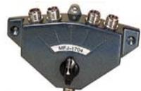
Antenna switching is an important part of any station and for low loss results you need a coaxial type. This one is a 4-way design with beautifully positive movement. SO-239 DC-500MHz, 2kW and up to 60dB isolation.
