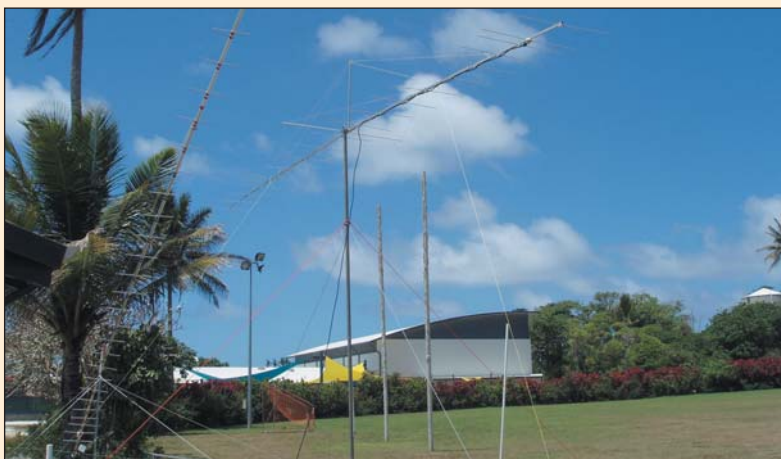
The antenna farm used by Rex Moncur, VK7MO, during his VK9XMO EME operation on 2m and 70cm from Christmas Island. The 70cm Yagi was assembled on site using insulation tape and the desired elevation was achieved by a shopping bag filled with sand hanging off the back end.
