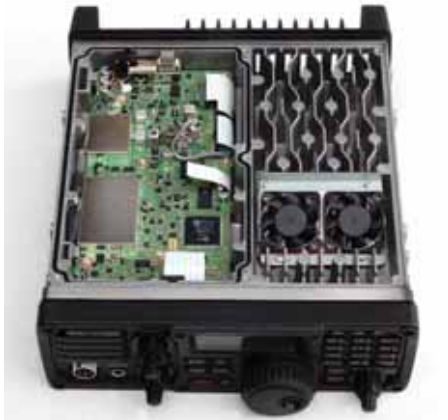
Opening the top cover reveals the main PCB and substantial fan-blown heatsink.
