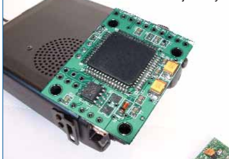
PHOTO 1: Speech intelligibility measurement allows noise filters like this one from bhi to be evaluated objectively.
