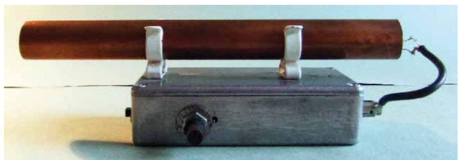
PHOTO 2: The receiver uses a length of tube to shield the phototransistor from extraneous light.
