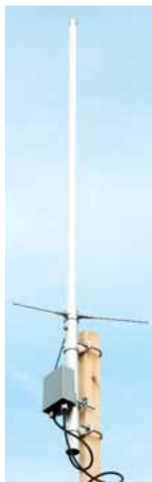
The antenna that was mounted as high as possible for best results.
