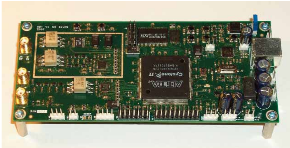
The All Digital Transceiver is a compact single board design.
