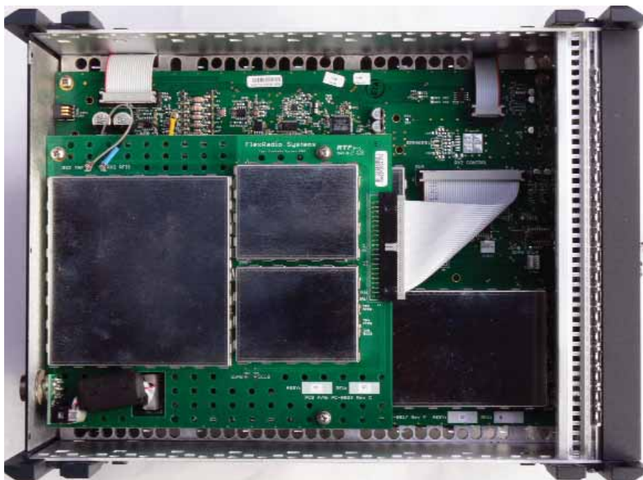
Second receiver mounted on the main board. Assembly and connection is very easy.
