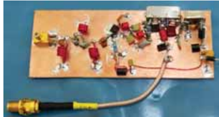
PHOTO 1: With only a little effort it's possible to make a converter to receive the 60MHz and 70MHz beacons.
