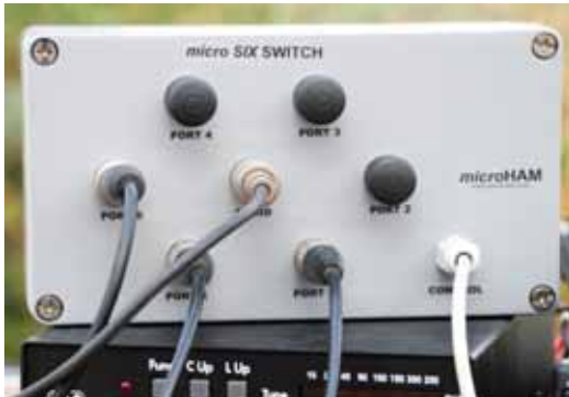
PHOTO 4: Each SO239 is numbered and the antenna connected to that port must relate to the same antenna port in the software.
