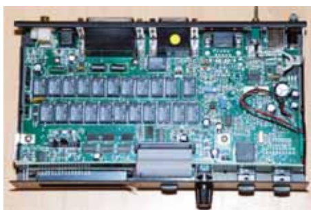
PHOTO 1: Matching the Station Master to your rig entails removing the top case and setting a series of jumpers as explained in the manual to get them talking to each other.
