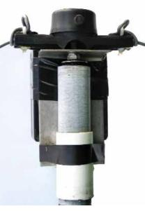
PHOTO 3: Close-up of the rotating dipole centre (balun box to the rear).
