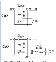
FIGURE 1: DC injector/extractor. (a) Basic circuit, (b) With optional extras [1].
